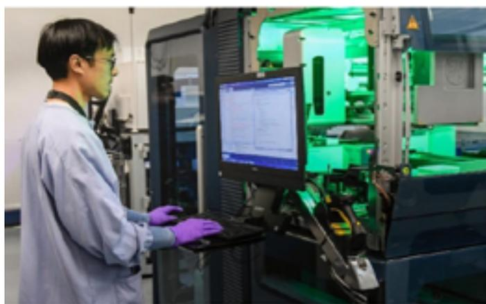
Spencer Trinh replicates the fraction library onto 384 well plates on the Hamilton Microlab Vantage Liquid Handler to be sent to screening centers around the world.
