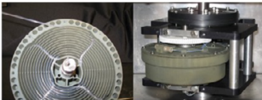
FIG. 3 Cross-section of spiral tubing support rotor with circular channels and 4 radial channels where tubing is guided in 4 loops per layer. Assembled rotor with top and tubing connected to flow tubing that enters shaft and out center axis.
